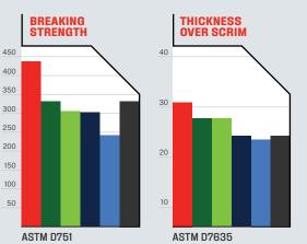
Based on published ASTM data for breaking strength and thickness over scrim posted on competitor websites using 60 mil PVC as the benchmark. For additional Elevate MAX PVC and Elevate MAX PVC XR ASTM results, please refer to the Technical Information Sheet on holcimelevate.com.
